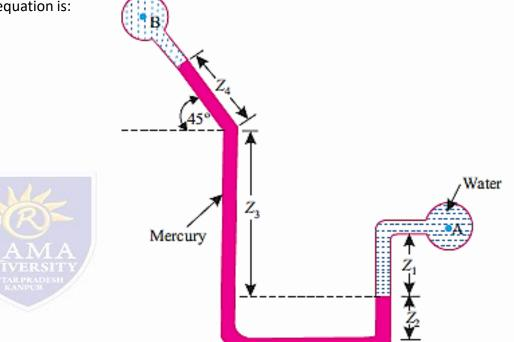
• From the Fig. 2.30 determine the absolute pressure in pipe A that contains oil of specific gravity = 0.88. Take Z1 = 0.66 m, Z2 = 0.33 m, Z3 = 0.165 m and Z4 = 0.11 m. Assume an atmospheric pressure 105 kPa.
